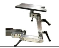
10. Each locking lever, when loosened, permits its pin to rotate. Thus each locking lever enables its subsequent part (link, knuckle, or stub shaft) to rotate 360 degrees. Loosening only one locking lever enables freedom at only a single joint of the articulating work rest system. Loosening two locking levers at the same time enables two joints to move freely. Loosening three locking levers at the same time enables three joints to move freely.
