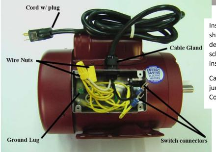
Install the power cord with the cable gland as shown in the photo. Connect the wires as detailed in the wiring diagram / switch schematic. Note the grounding lug located inside the junction box.
