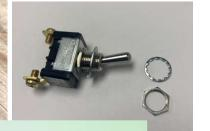
The switch is notched so that the "off" part of the switch is down and aligned with both the tooth on the junction box cover and the tooth in the switch guard. The switch fasteners should be attached as follows: first a hex nut, then the spacing ring, then penetrate the junction box cover, then the switch guard, then the toothed locking ring, finally a hex nut for tightening.
