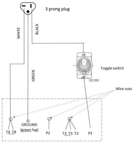
MOTOR WIRE NUMBERS for 110089 1-1/2 hp motor HIGH VOLTAGE (208-230 volts)
