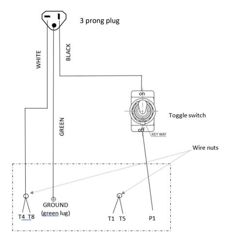
MOTOR WIRE NUMBERS for 110090 2 HP motor 230 VAC SINGLE PHASE INPUT
